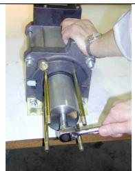
Tighten the castle groove with 25 Nm. The piston sealing ring is pushed onto the O ring during tightening.
