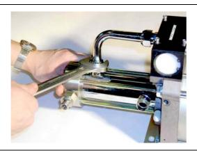
Loosen the cooling pipe union nuts from pilot valve to cooling cylinder.
