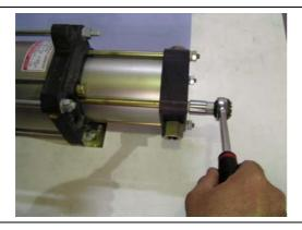
Loosen the four hexagon nuts from the stud bolts.
