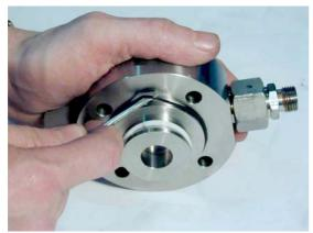
Remove the O ring that seals the cooling cylinder.
