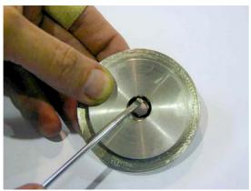
Remove the O ring from the HP piston.
