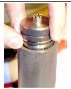
Insert the complete sub-assembly into the pressure cylinder. Check the correct seat of the guiding ring in the groove.
