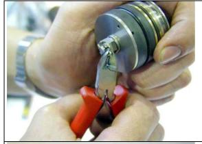
Remove the retaining pin.
