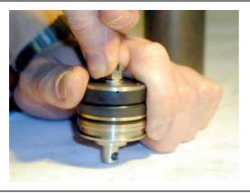
Compress the complete sealing package in anti-spring force direction. For the time being, tighten the castle nut only slightly (2-3 thread turns).
