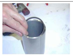
Insert the piston sealing ring into the HP cylinder and align the ring parallel ca. 13 mm below the cylinder edge.
