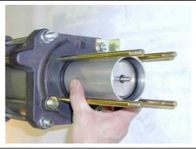
Push the HP cylinder over the HP piston until the piston sealing ring fits close to the O ring.
