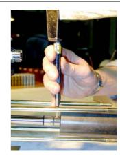
Push the securing sleeve over the securing pin and safeguard it with the O ring.
