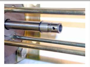
Attach the dowel pin and insert the centring piston into the boring at the piston rod, then beat in the dowel pin.
