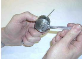
Carefully loosen the castle nut. Caution: Tightened package expands due to spring pretensions.
