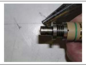
Remove the retaining pin.
