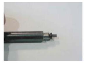
Slip the serrated ring, washer and O ring in this order onto the centring mandrel. When attaching the serrated ring, make sure that the serration points away from the O ring.
