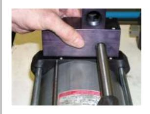
Re-attach the servo-valve with cooling tube and the air pipe, check the correct seat of the O rings.
