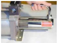
Loosen the HP cylinder by means of light taps with a plastic hammer from the top cover.
