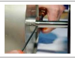
Safeguard the sub-assembly with the retaining pin.
