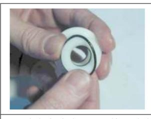
Then mount the two O rings into the grooves at the external diameter of the bushing.
