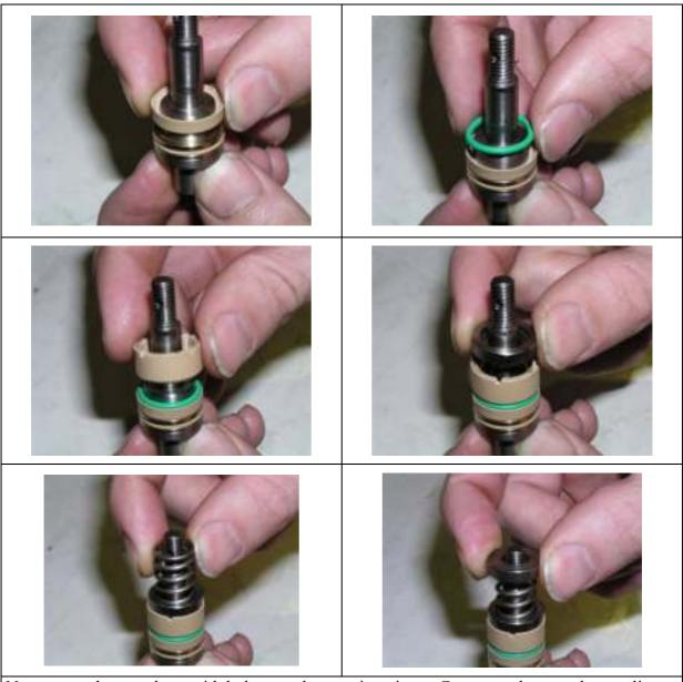
Now screw the round nut with hole onto the centring piston. Compress the complete sealing package in anti-spring force direction until the two borings (round nut with hole and centring piston) are aligned.
