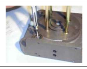
Withdraw the USIT ring, compression spring and pilot valve tappet.
