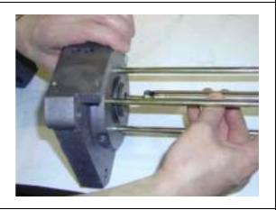
Insert the piston rod into the piston rod holder of the air pistons and fasten with the pin.
