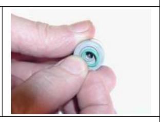
Remove the valve seat, spring and ball from the valve body.
