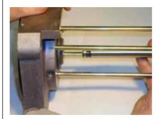
Pull the piston rod out of the top cover into the direction of the HP part.
