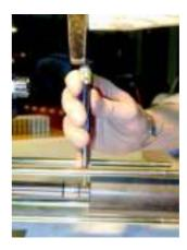
Push the securing sleeve over the securing pin and safeguard it with the O ring.
