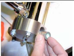
Screw the inlet and outlet sockets into the HP head and tighten the sockets with 120 Nm.
