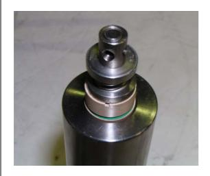
Insert the complete sub-assembly into the pressure cylinder.
