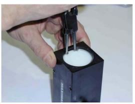
Dismantle the locking ring at the spool valve housing with suitable locking ring pliers. (The ring is located opposite the compressed air inlet).
