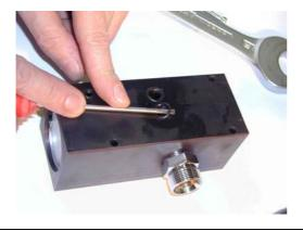
Remove the O rings that seal the top cover.
