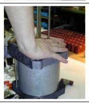
Carefully push the air drive part together until the air cylinder fits closely to the top cover.
