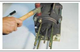
The DLE is placed on a workbench for alignment and a soft hammer is used to align the top and bottom cover in parallel.
