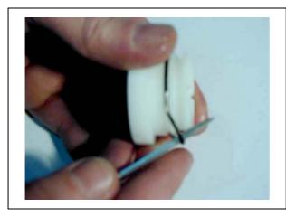
Remove the O ring from the sealing cap.
