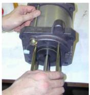
Slightly push the top and bottom cover together and insert the capillary control tube.
