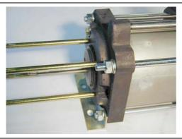
Also on the opposite side, the fastening brackets, screw retainers and washers are preassembled together with the hexagon nuts.
