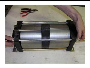
Remove the four hexagon nuts from the hexagon bolts.
