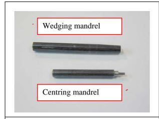
The following tools are necessary to reassemble the pilot valves: A centring mandrel, Works No. 3610.0284, and a wedging mandrel Works No. 3610.0285
