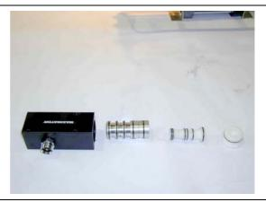
Remove the O rings from the spool and, if applicable, from the spool valve sleeve.
