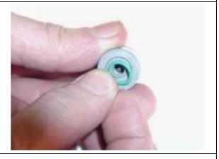
Remove the valve seat, spring and ball from the valve body.
