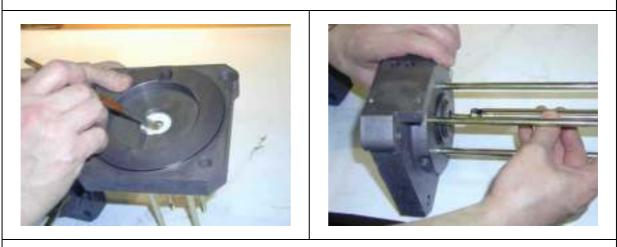
Insert the piston rod into the piston rod holder of the air pistons and fasten with the pin.
