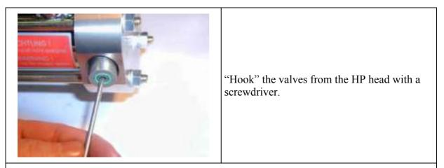
Remove the two O rings from the valve body.
