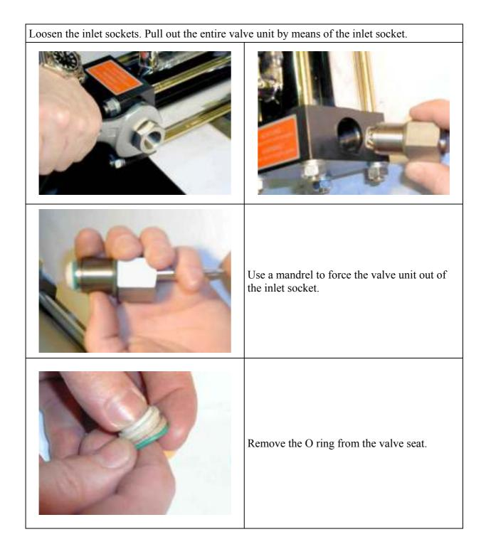
Remove the O ring from the inlet socket.
