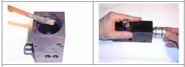
Re-insert the sealing cap into the spool valve housing and fasten it with the locking ring.
