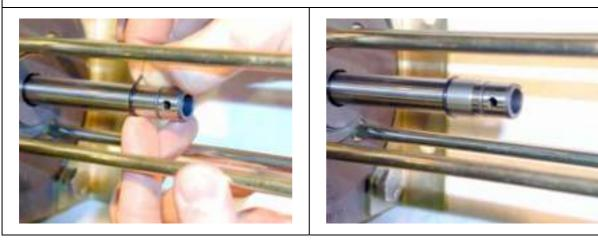
Attach the dowel pin and insert the centring piston into the boring at the piston rod, then beat in the dowel pin.
