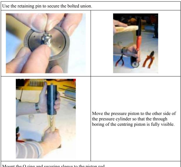
Mount the O ring and securing sleeve to the piston rod.
