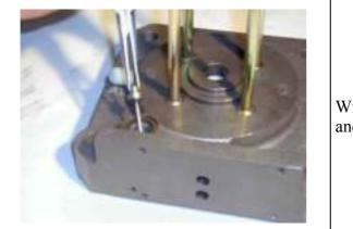
Withdraw the USIT ring, compression spring and pilot valve tappet.
