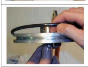
Remove the O ring from the air piston.
