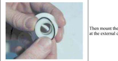
Then mount the two O rings into the grooves at the external diameter of the bushing.
