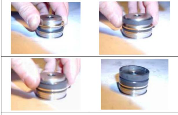
Grease the centring piston and attach its pertaining spring.
