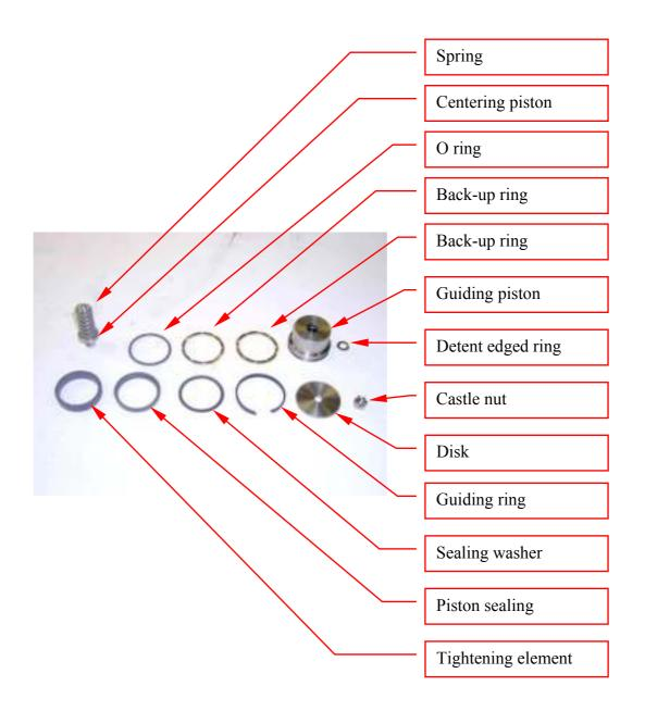
Remove the O ring and the back-up ring with a screwdriver from the guiding piston.
