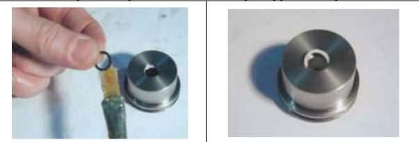
Put the following on the guiding piston in the indicated sequence: Sealing washer, back-up ring, piston packing, O ring (well greased) and tightening element.
