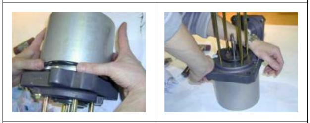
Carefully move the piston rod from outside through the greased bearing bush of the top cover. Caution: Make sure not to damage the sliding rings in the bearing bush in the process.
