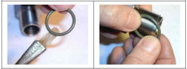
Grease the O ring that seals the valve seat and insert the ring in to the HP head.
