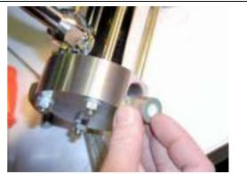
Screw the inlet and outlet sockets into the HP head and tighten the sockets with 120 Nm.
