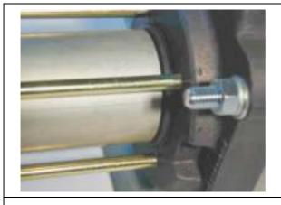
Push the HP cylinder over the O ring of the top cover till to the stopper. Caution: Make sure not to damage the O ring.
