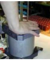
Carefully push the air drive part together until the air cylinder fits closely to the top cover.
