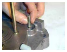
Slip the compression spring onto the pilot valve tappet.
