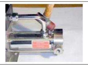
Carefully separate the compressor head by means of light taps with a plastic hammer from the HP cylinder.
