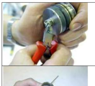
Remove the retaining pin.
