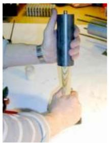
Move the pressure piston to the other side of the pressure cylinder so that the through boring of the centring piston is fully visible.
