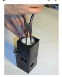
Use a small quantity of grease to "glue" the O rings for the sealing between spool valve housing and top cover into the O ring nests.
