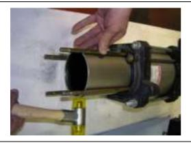
Loosen the HP cylinder by means of light taps with a plastic hammer from the top cover.
