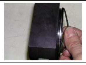
Remove the O rings of the HP head.
