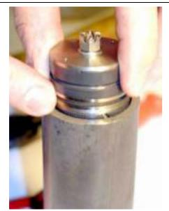
Insert the complete sub-assembly into the pressure cylinder. Check the correct seat of the guiding ring in the groove.
