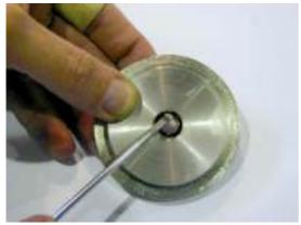
Remove the O ring from the HP piston.
