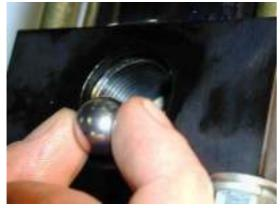
Insert the ball into the valve seat.
