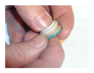
Remove the O ring from the valve seat.
