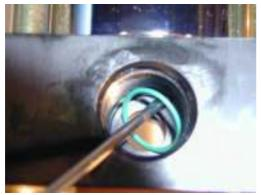
Remove the O ring that seals the valve seat.
