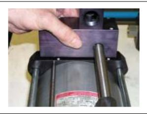
Re-attach the spool onto the DLE. During the process, guide the air pipes into the spool valve housing.
