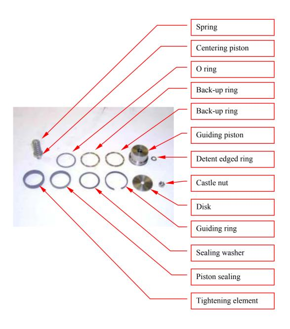
Remove the O ring and the back-up ring with a screwdriver from the guiding piston.
