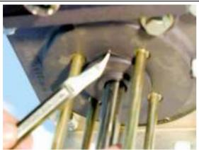
Dismantle the O rings that seal the cooling cylinder and the HP cylinder.
