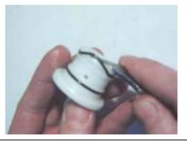
Remove the O rings from the bearing bush.
