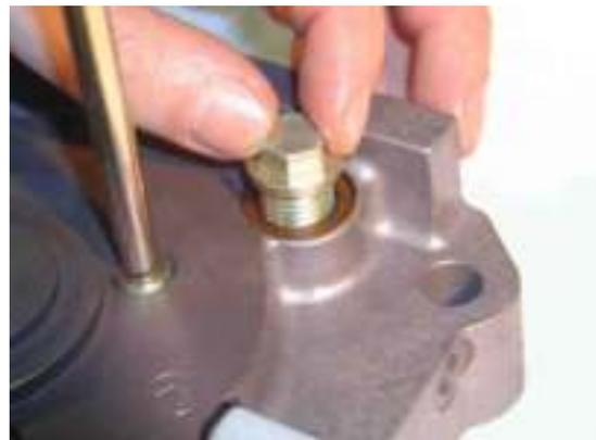
Now turn the top cover round. Then use the wedging mandrel to safeguard the serrated ring against slipping out. Upset the boring with a few hammer strokes.
