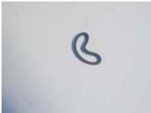
Form the sliding ring into a kidney shape and insert it. Subsequently, bring the sliding ring inside the groove back into its original form. Caution: Do not bend the sliding ring too sharply.
