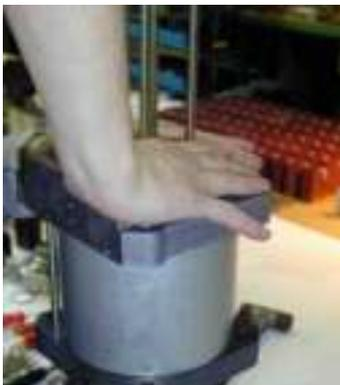
Carefully push the air drive part together until the air cylinder fits closely to the top cover.
