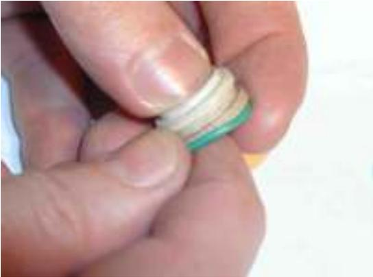
Remove the O ring from the valve seat.
