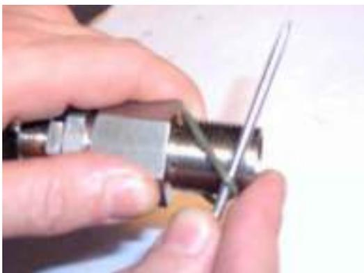
Remove the O ring from the outlet socket.
