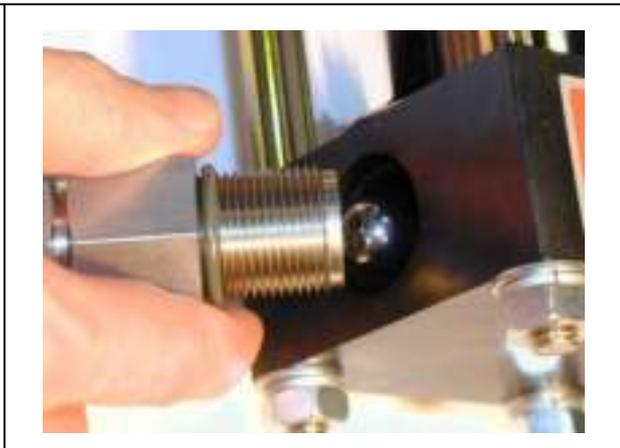
Use a mandrel to force out the valve seat, that is still in the HP head.
