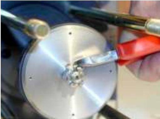
Remove the retaining pin of the castle nut.
