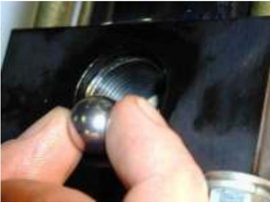
Insert the ball into the valve seat.
