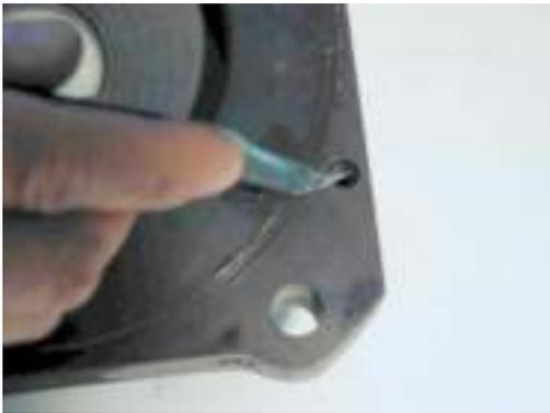
Dismantle the O rings for the control pipe from the top and bottom covers.
