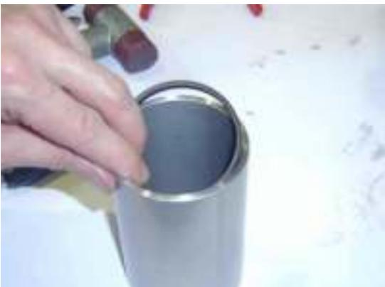
Insert the piston sealing ring into the HP cylinder and align the ring parallel ca. 13 mm below the cylinder edge.
