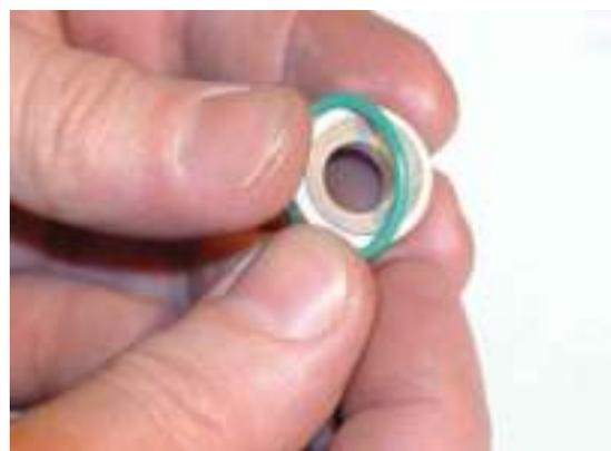
Place the valve seat and the ball onto the inlet socket and carefully press them into the socket.
