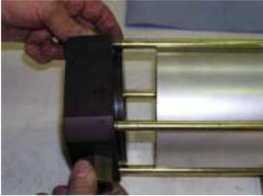
Push the compressor head over the stud bolts. Make sure that the suction and pressure lines can be mounted without any warping.
