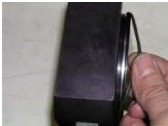
Remove the O rings of the HP head.
