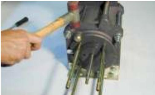
The DLE is placed on a workbench for alignment and a soft hammer is used to align the top and bottom cover in parallel.
