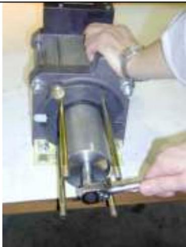
Tighten the castle groove with 25 Nm. The piston sealing ring is pushed onto the O ring during tightening.
