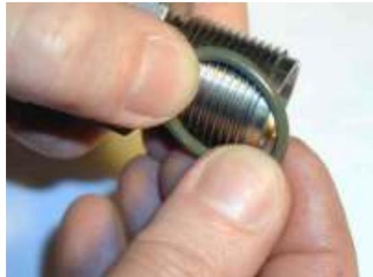
Grease the O ring that seals the valve seat and insert the ring in to the HP head.
