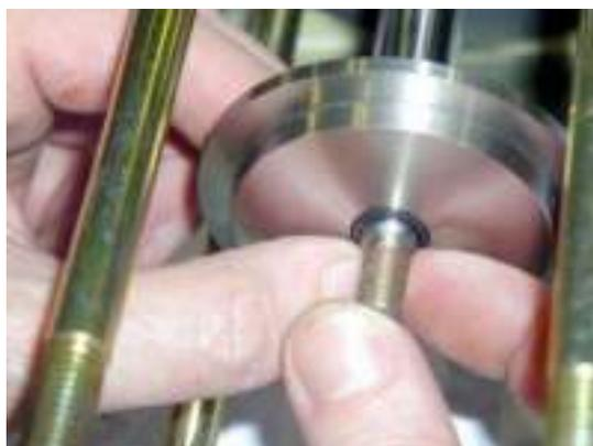
Grease the O ring and mount it into the HP piston.
