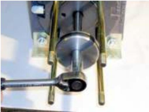
Loosen the castle nut. If the HP piston follows to turn, it is recommended to use an impact screwdriver to loosen the castle nut.
