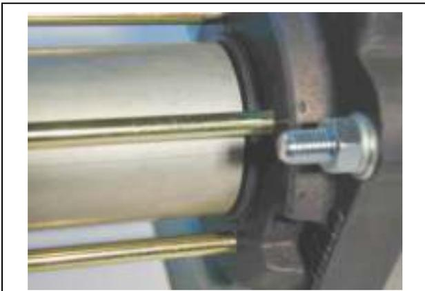
Push the HP cylinder over the O ring of the top cover till to the stopper.
