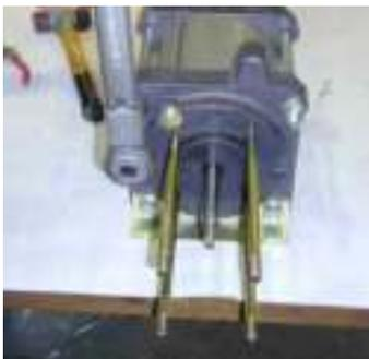
Then tighten the hexagon nuts crosswise with the specified torque of 55 Nm.
