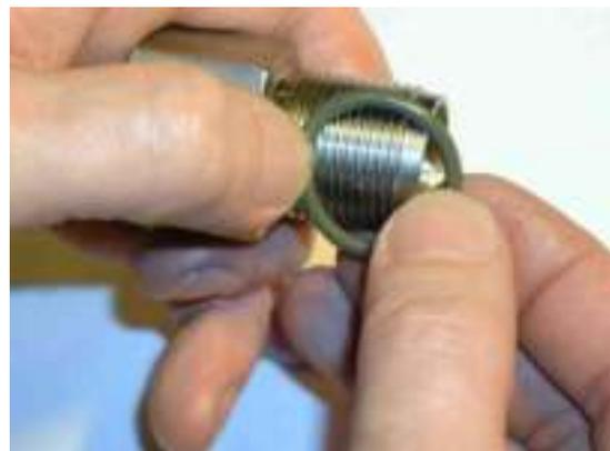
Grease the O ring that seals the valve seat and slip it onto the valve seat.
