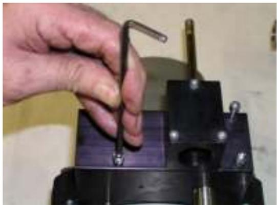
Place the 4 socket head screws to fasten the spool valve housing and tighten the screws with 5 Nm.
