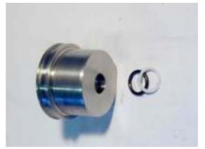
Dismantle the two back-up rings and the O ring from the HP head.
