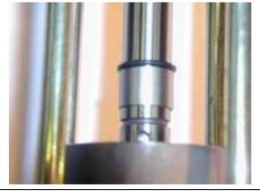
Move the O ring and the securing sleeve along the piston rod until the boring for the dowel pin is free.
