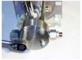
Loosen the four hexagon nuts from the stud bolts.
