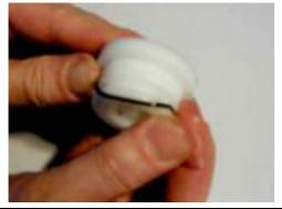
Slip the O rings onto the servo-valve, sealing cap and, if applicable, the spool valve sleeve.
