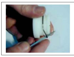
Remove the O ring from the sealing cap.
