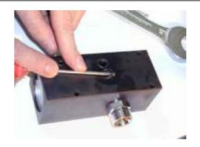
Remove the O rings that seal the top cover.
