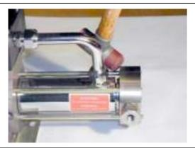
Carefully separate the compressor head by means of light taps with a plastic hammer from the HP cylinder.
