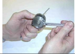
Carefully loosen the castle nut. Caution: Tightened package expands due to spring pretensions.
