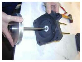
Insert the air piston with piston rod into the bottom cover.
