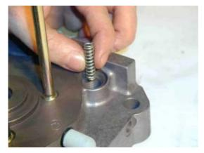
Slip the compression spring onto the pilot valve tappet.
