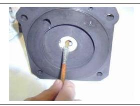
Grease the bearing bush of the bottom cover.
