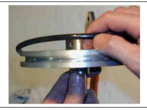
Remove the O ring from the air piston.
