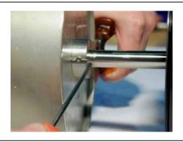
Safeguard the sub-assembly with the retaining pin.
