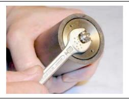
Tighten the castle groove with the specified torque of 20 Nm.
