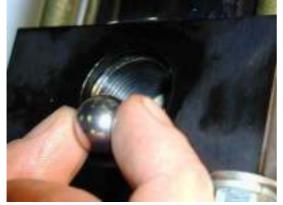
Insert the ball into the valve seat.
