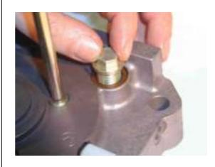
Now turn the top cover round. Then use the wedging mandrel to safeguard the serrated ring against slipping out. Upset the boring with a few hammer strokes.
