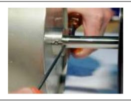
Safeguard the sub-assembly with the retaining pin.
