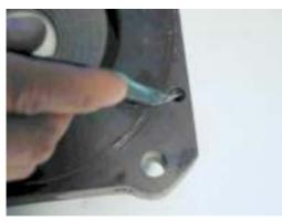
Dismantle the O rings for the control pipe from the top and bottom covers.
