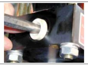
Use a cone-shaped mandrel to force the valve seat into the HP head.
