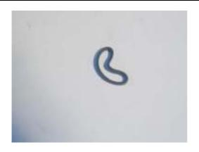
Form the sliding ring into a kidney shape and insert it. Subsequently, bring the sliding ring inside the groove back into its original form. Caution: Do not bend the sliding ring too sharply.
