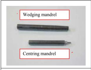
The following tools are necessary to reassemble the pilot valves: A centring mandrel, Works No. 3610.0284, and a wedging mandrel Works No. 3610.0285
