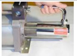
Loosen the HP cylinder by means of light taps with a plastic hammer from the top cover.
