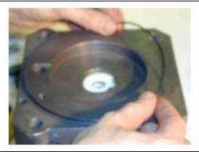
Mount the O ring that seals the air cylinder.
