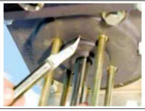
Dismantle the O rings that seal the cooling cylinder and the HP cylinder.
