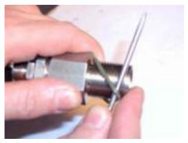
Remove the O ring from the outlet socket.
