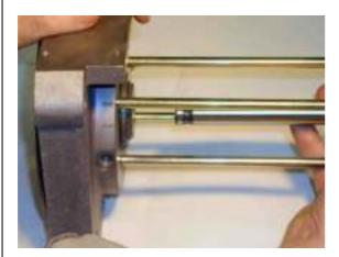
Pull the piston rod out of the top cover into the direction of the HP part.
