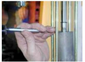
Use a suitable mandrel to drive the dowel pin Item 16 out of the boring.
