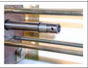
Attach the dowel pin and insert the centring piston into the boring at the piston rod, then beat in the dowel pin.
