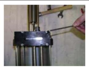
Place the 4 socket head screws to fasten the spool valve housing and tighten the screws with 5 Nm.
