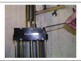
Loosen the socket head screws in the spool valve housing.
