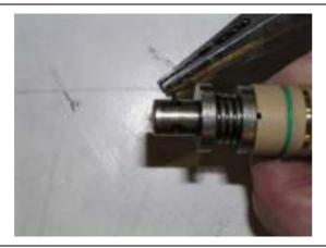
Remove the retaining pin.
