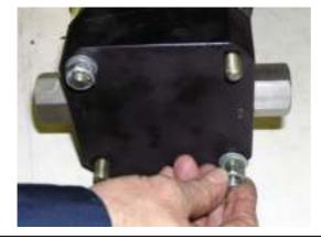
Attach the hexagon nuts and screw retainers to the stud bolts. (Do not tighten!)
