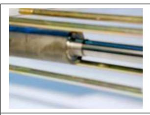
Push the HP piston in the direction of the second stage until the stop point. Draw the HP cylinder from the HP piston until it levels with the former.
