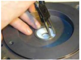
Insert the locking ring into the foreseen groove. Check also for its correct seat.
