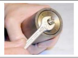
Tighten the castle groove with the specified torque of 20 Nm.
