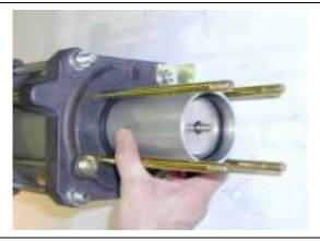
Push the HP cylinder over the HP piston until the piston sealing ring fits close to the O ring.
