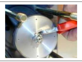
Remove the retaining pin of the castle nut.
