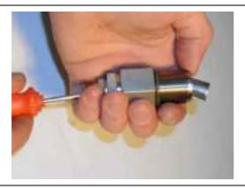
Force the ball holder out of the outlet socket.
