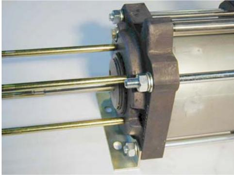
Also on the opposite side, the fastening brackets, screw retainers and washers are pre-assembled together with the hexagon nuts.
