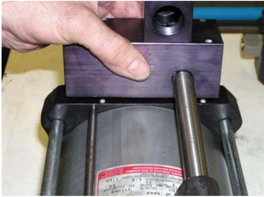
Re-attach the servo-valve with cooling tube and the air pipe, check the correct seat of the O rings.
