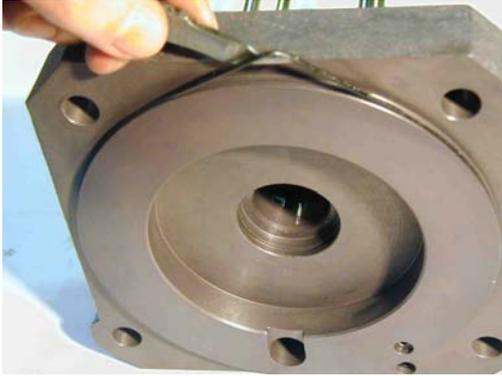
Dismantle the O ring that seals the air cylinder.
