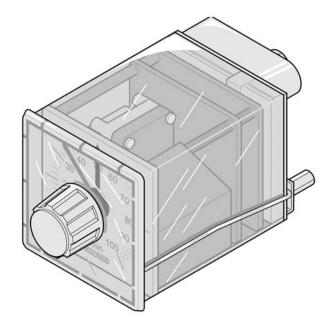
The 54 Series timer is a totally pneumatic device with +/-1% repeatability. Timing is fully adjustable throughout the timing range by a knob on the front dial face. The standard timer is equipped with a special 4 way valve which provides for on or off delay timing (depending on plumbing connections). The front dial displays set time and the time remaining in the cycle.
