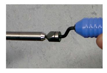
The only work left to do now is debur-ring of the internal diameter of the finished pipe. Carefully remove all chips that are generated by taper cutting edges and deburring (inside and out-side).
