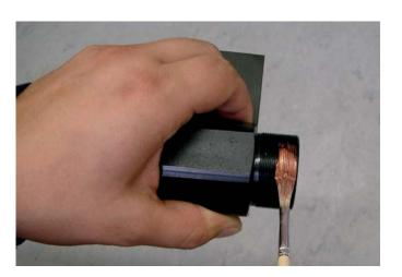
Lubricate the threads of knurled nut and base structures (We recommend use of solid lubricant. such as copper paste).
