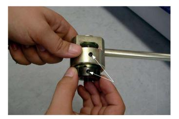
Insert the die stock and guide bush into the tool body and secure with headless set screws. Align the components in such a manner that the headless set screws grip into the recesses.
