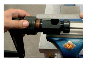
Turn out the knurled screw until only approx. 2-3 thread turns are gripping. This corresponds to a distance of 20 mm between knurled nut and the step of the base structures.
