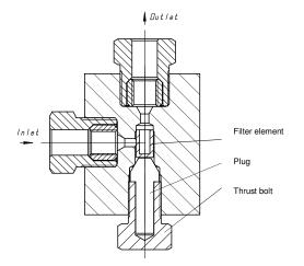
Figure 15: Structure of a angle filter
