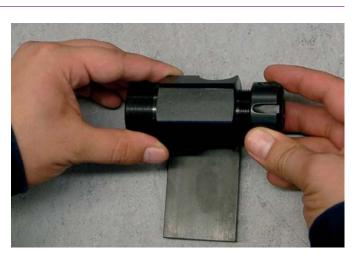
Push the collet chuck into the tensioning nut.
