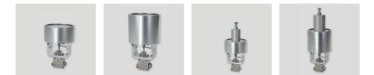
MAXIMATOR air operated valve actuators are piston type design, and are mounted on a manual valve to provide remote control capability. There are two air to open actuators and two air to close actuators available, and selection is based on the valve size, system pressure, and air pressure available.
