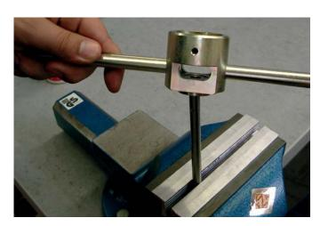
Place the threading tool with guide bush on top of the tube.
