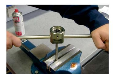
Slightly press down the tool and start the threading operation (in counter-clockwise direction). Rotate the tool briefly in clockwise direction during the threading process in order to break the chip and apply more cutting oil.
