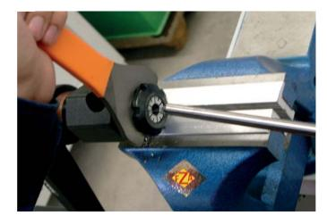
Use the chuck key to loosen the tensioning nut and the tube can be re-moved from the coning tool.
