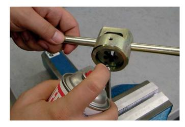
Wet the pipe and the die with cutting oil.
