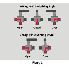
Ball valves are available as 2-way and 3-way model and are designed for closing/opening applications. The 3-way model is also available as a 90° switch and also 180° switch version (middle setting closed) (see also Fig.3). Compared to 2-part stem, ball valves with trunnion mounted, single-part valve stems prevent shear fracture and also reduce the impact of lateral forces.
