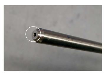
The finished pipe can be recognised by the completely machined face side of the pipe. The taper surface must be free from any damage, such as indentations or scratches. If this is not the case, the pipe can simply be re-cut.
