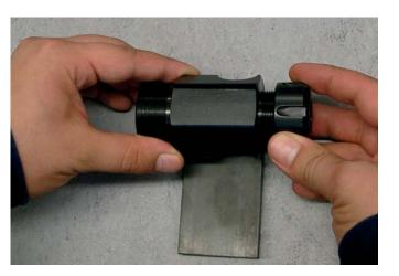
Slightly grease tensioning nut and collet chuck and screw them onto the base structure.
