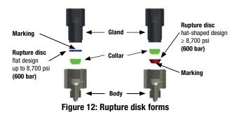
The tightening torque for the hold-down nut based on a thread treated with lubricant paste is indicated on the rupture disk type label. Figure 12 shows the two rupture disk forms. This is a flat or hat-shaped rupture disk that can be used depending on the pressure requirements.
