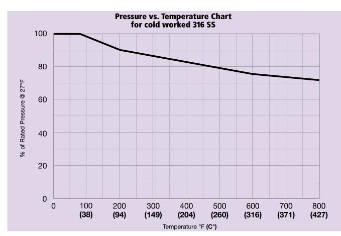
Note: The above pressure temperature chart is for 316 cold worked materials, this chart does not account for the temperature rating of packing or o-ring material which could be the limiting factor. Contact factory for other material limitations.
