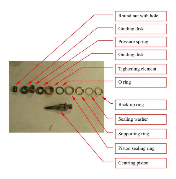
Dismantle the two back-up rings and the O ring from the HP head.
