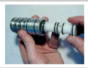
If applicable, grease the spool valve housing internally and install the spool valve sleeve with slight rotating motions into the spool valve housing.
