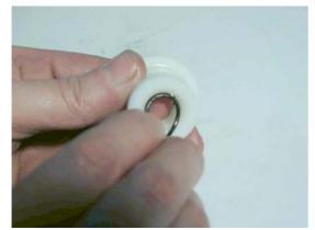
Insert the O ring into the bearing bush.
