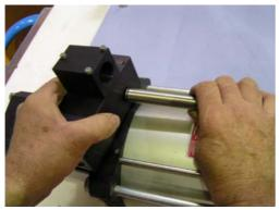
The air pipes are only loosely pushed in and can smoothly be withdrawn from the spool valve housing and the intermediate cover.
