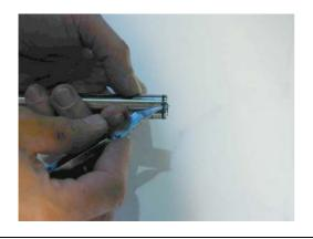
Remove the O rings from the pressure pipe.
