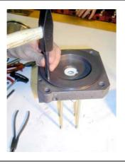
To begin with, insert the centring mandrel into the tappet boring. Then drive the entire package with some hammer strokes into the boring.
