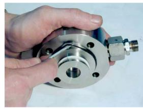
Remove the O ring that seals the cooling cylinder.
