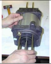
Slightly push the top and bottom cover together and insert the capillary control tube.
