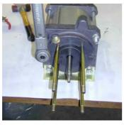
Then tighten the hexagon nuts crosswise with the specified torque of 55 Nm.
