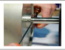
Safeguard the sub-assembly with the retaining pin.
