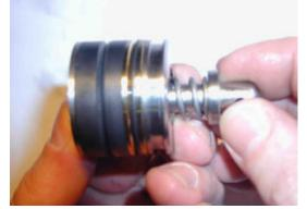
Place the disk on the tightening element and insert the centring piston into the guiding piston.
