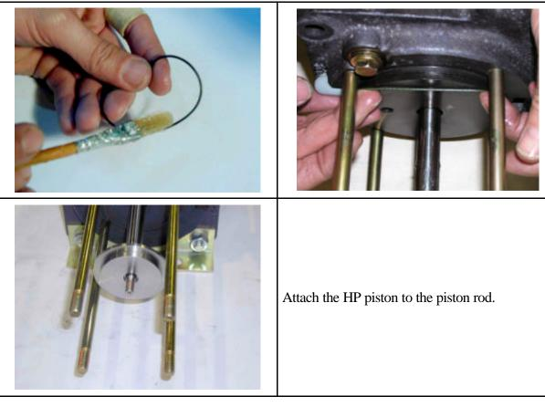
Grease the O ring and insert it into the groove between HP piston and piston rod.
