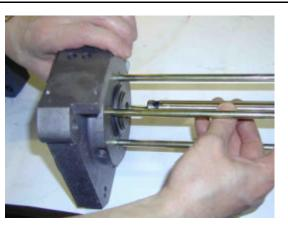
Insert the piston rod into the piston rod holder of the air pistons and fasten with the pin.
