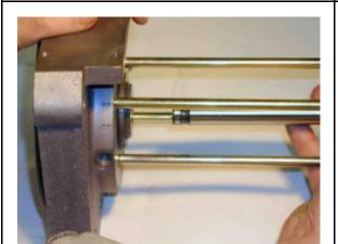
Pull the piston rod out of the top cover into the direction of the HP part.
