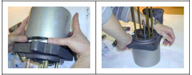
Carefully move the piston rod from outside through the greased bearing bush of the top cover. Caution: Make sure not to damage the sliding rings in the bearing bush in the process.
