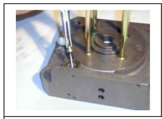
Withdraw the USIT ring, compression spring and pilot valve tappet.
