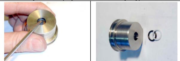
Dismantle the two back-up rings and the O ring from the HP head.
