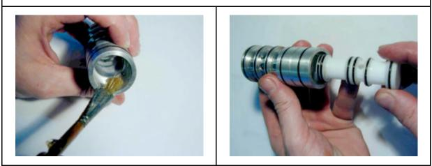
If applicable, grease the spool valve housing internally and install the spool valve sleeve with slight rotating motions into the spool valve housing.
