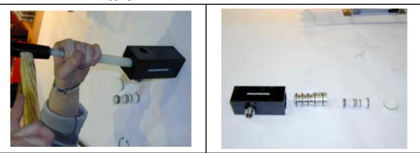
Remove the O rings from the spool and, if applicable, from the spool valve sleeve.
