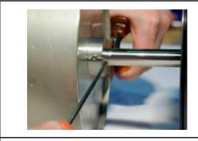
Safeguard the sub-assembly with the retaining pin.
