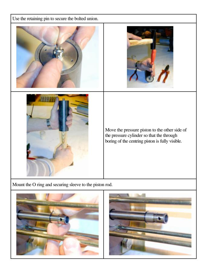
Attach the dowel pin and insert the centring piston into the boring at the piston rod, then beat in the dowel pin.
