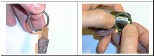
Grease the O ring that seals the valve seat and slip it onto the valve seat.
