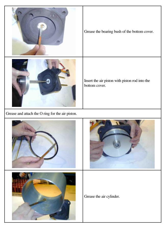
Attach the air cylinder onto the air piston, carefully insert the O ring into the cylinder while doing so. Push the air cylinder and the bottom cover together until the air cylinder fits closely to the bottom cover.
