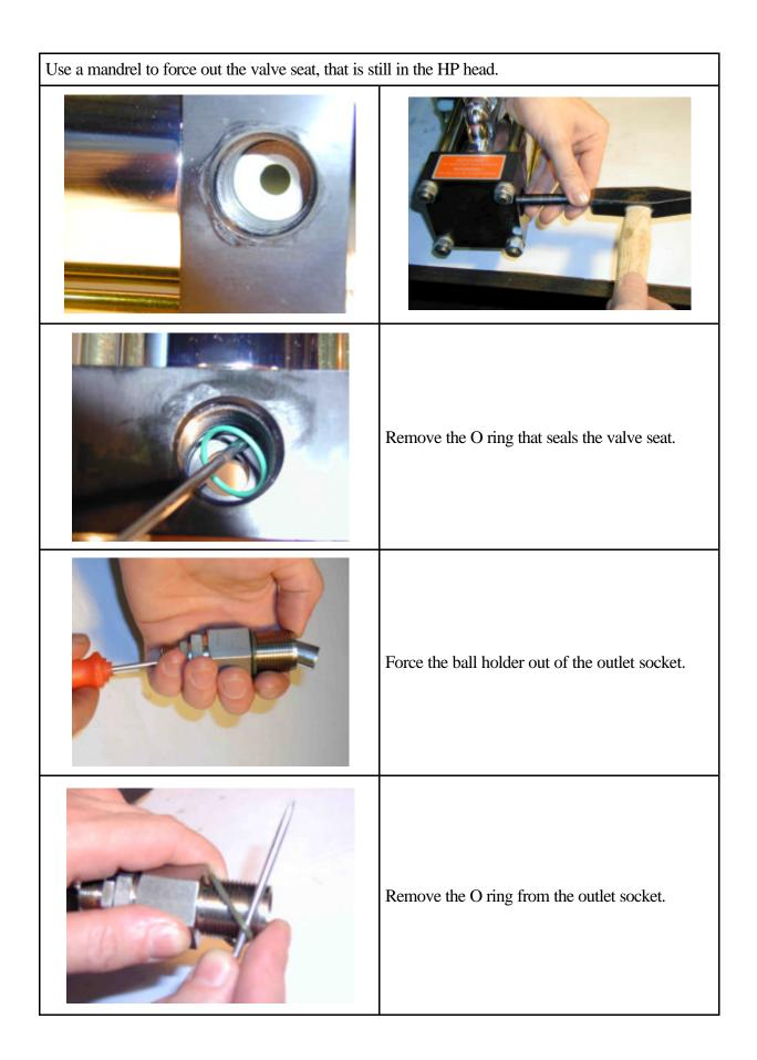
The main parts of the delivery valve are: Inlet socket, valve ball, spring, ball holder, valve seat and two O rings.
