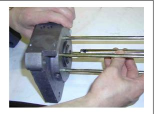
Insert the piston rod into the piston rod holder of the air pistons and fasten with the pin.
