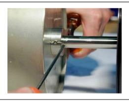
Safeguard the sub-assembly with the retaining pin.
