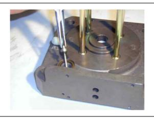
Withdraw the USIT ring, compression spring and pilot valve tappet.
