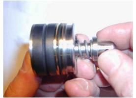
Place the disk on the tightening element and insert the centring piston into the guiding piston.
