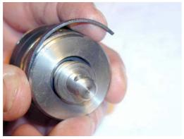
Place the guiding ring onto the guiding piston.
