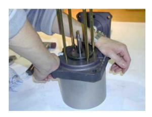
Carefully move the piston rod from outside through the greased bearing bush of the top cover. Caution: Make sure not to damage the sliding rings in the bearing bush in the process.
