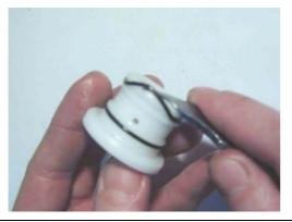
Remove the O rings from the bearing bush.
