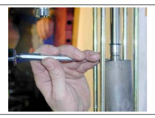
Use a suitable mandrel to drive the dowel pin Item 16 out of the boring.
