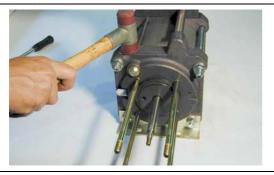
The DLE is placed on a workbench for alignment and a soft hammer is used to align the top and bottom cover in parallel.
