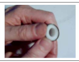
Grease the spool valve sleeve well, even when it is still installed. Insert the spool with rotating motions into the spool valve sleeve.
