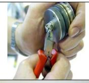
Remove the retaining pin.
