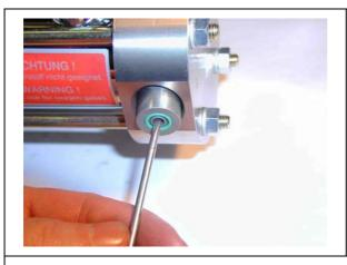
"Hook" the valves from the HP head with a screwdriver.
