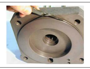
Dismantle the O ring that seals the air cylinder.
