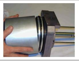
Withdraw the air cylinder from the top cover and the air piston.
