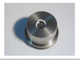
Put the following on the guiding piston in the indicated sequence: Sealing washer, back-up ring, piston packing, O ring (well greased) and tightening element.
