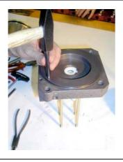
To begin with, insert the centring mandrel into the tappet boring. Then drive the entire package with some hammer strokes into the boring.
