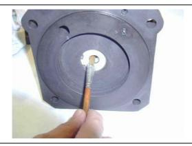
Grease the bearing bush of the bottom cover.
