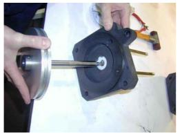
Insert the air piston with piston rod into the bottom cover.
