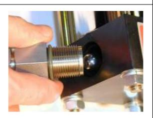
Use a mandrel to force out the valve seat, that is still in the HP head.
