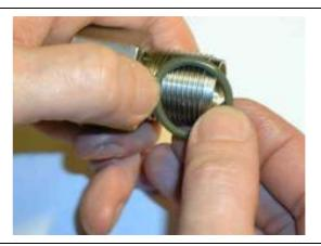
Grease the O ring that seals the valve seat and slip it onto the valve seat.
