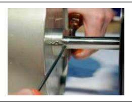
Safeguard the sub-assembly with the retaining pin.
