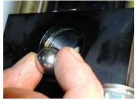
Insert the ball into the valve seat.
