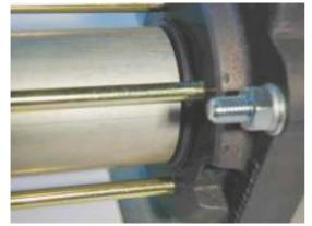
Push the HP cylinder over the O ring of the top cover till to the stopper.
