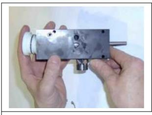
Use a mandrel to force out the spool valve sleeve with light strokes of the spool valve housing.
