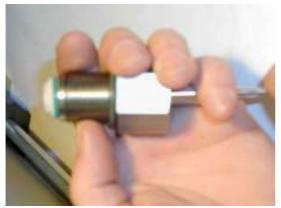
Use a mandrel to force the valve unit out of the inlet socket.
