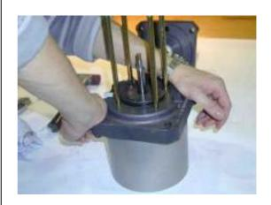
Carefully move the piston rod from outside through the greased bearing bush of the top cover. Caution: Make sure not to damage the sliding rings in the bearing bush in the process.
