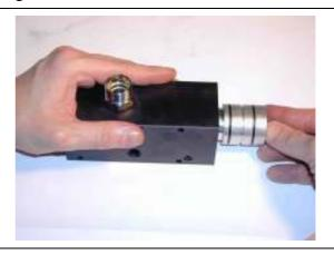
Re-insert the sealing cap into the spool valve housing and fasten it with the locking ring.
