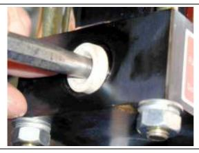
Use a cone-shaped mandrel to force the valve seat into the HP head.
