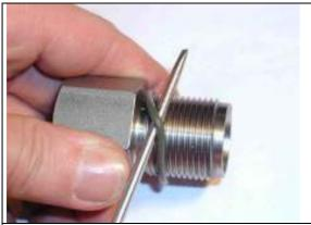
Remove the O ring from the inlet socket.
