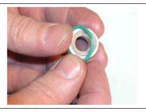
Place the valve seat and the ball onto the inlet socket and carefully press them into the socket. Place the spring on top of the ball. Slip the ball holder over the spring.
