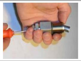
Force the ball holder out of the outlet socket.
