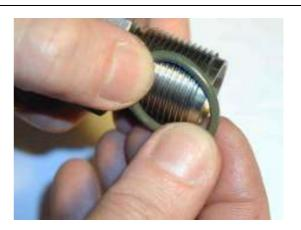
Grease the O ring that seals the valve seat and insert the ring in to the HP head.
