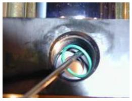
Remove the O ring that seals the valve seat.
