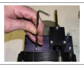
Loosen the socket head screws in the spool valve housing.
