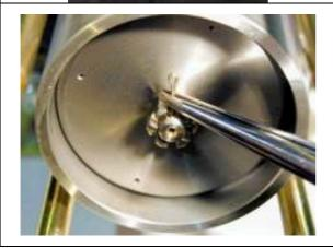
Use the retaining pin to secure the castle nut (appropriately bend the retaining pin with a screwdriver).
