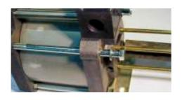
Attach washers and fastening brackets to the hexagon bolts and mount these assemblies. Caution: The hexagon bolt (longer design) is placed at the air supply side, marked with PL.
