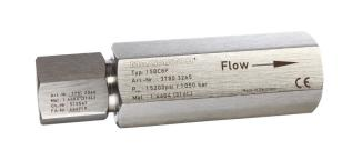
**MAXIMATOR** Pipe ball check valves prevent reverse flow where bubble tight shutoff is not mandatory. These check valves are designed to operate to 660°F. These check valves are not to be used as a relief device. The opening pressure of the pipe ball check valves is approximately 10 psi.
