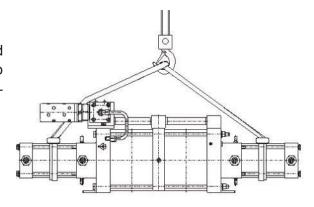
Fig. 8 DLE lifting points
