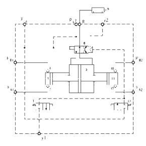
Fig. Connection diagram for double-acting booster
