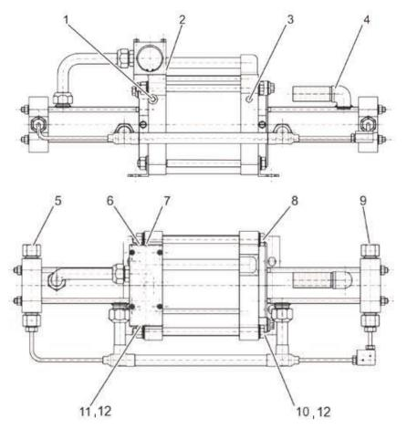
Fig. Ports for combined booster
