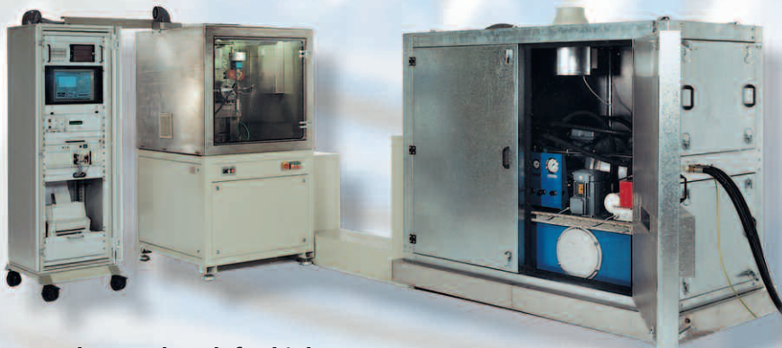
Pulse test bench for high-pressure components
