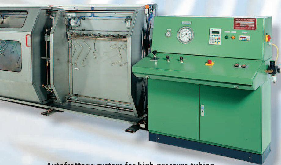
Autofrettage system for high-pressure tubing
