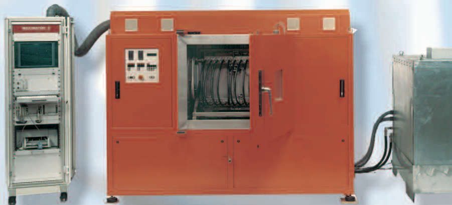
Pulse test bench for hose lines
