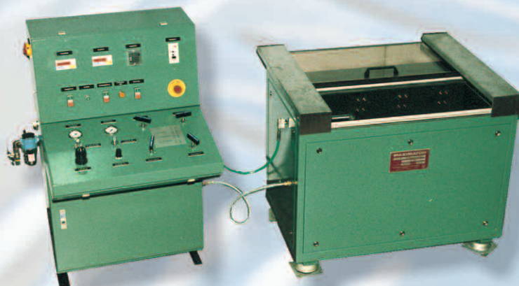
Bursting pressure test bench for air bag cold gas tank
