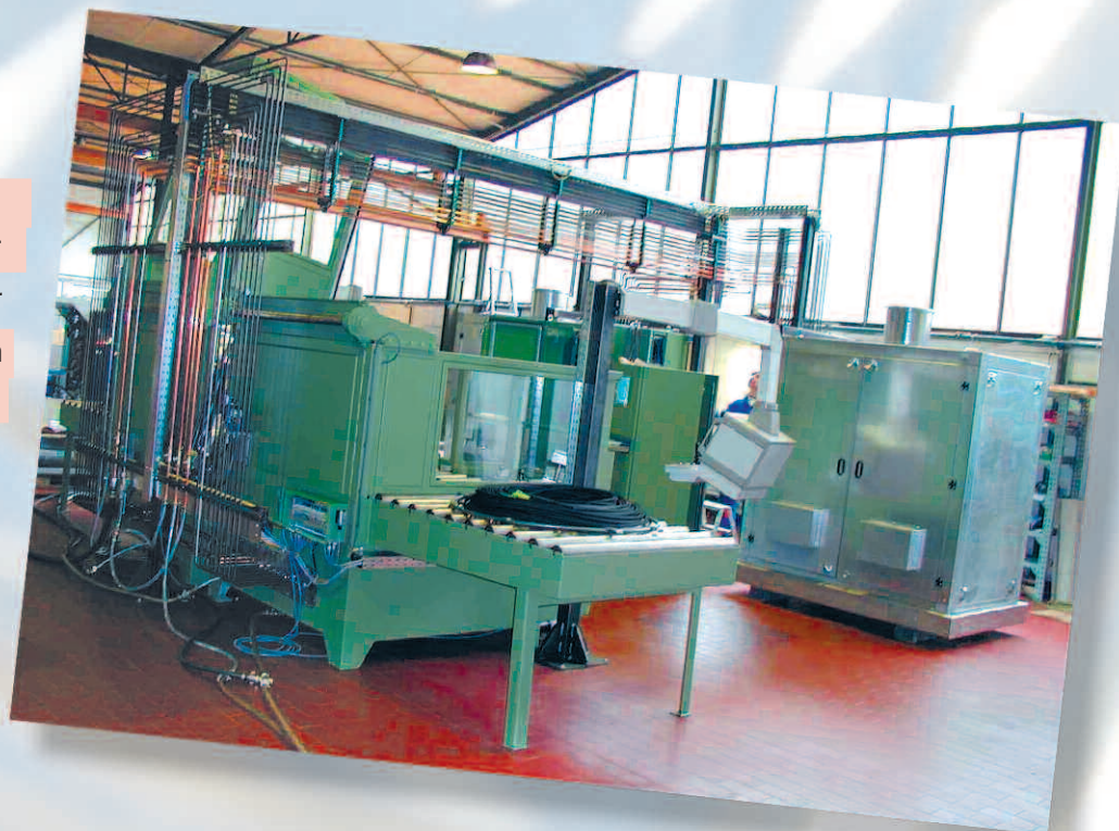
Mandrel extraction system for hose lines
