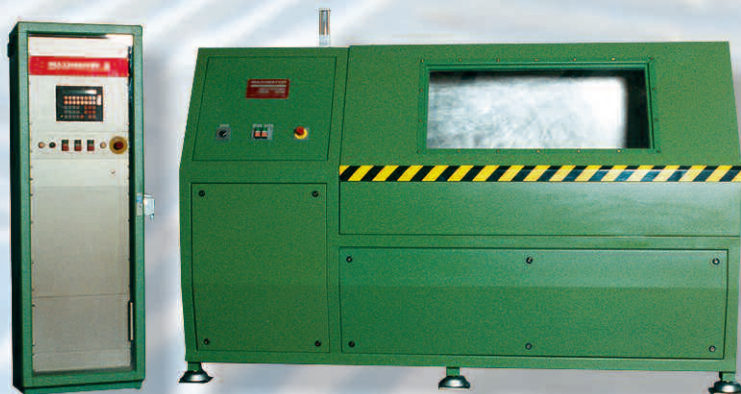
Bursting pressure test bench for undercarriage hoses
