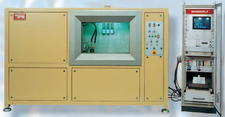
Pulse test bench for filter housings
