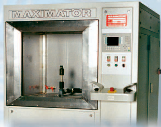
Autofrettage system for high-pressure loaded vehicle components
