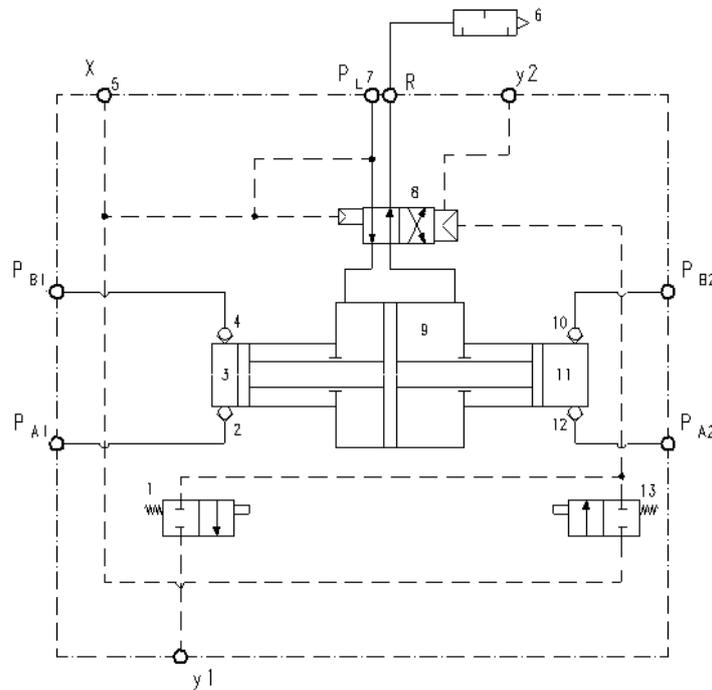
Fig. Circuit diagram of the booster
