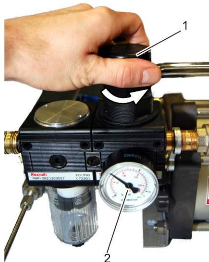
5. Open the venting screw (1) on the water separator (2) and release the water.
