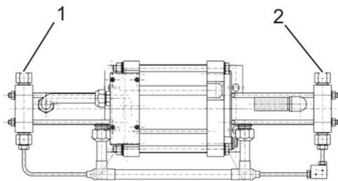
1. ➔ Remove the plug at the inlet and outlet ports (1 and 2).
