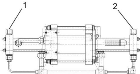
1. ➔ Remove the plug at the inlet and outlet ports (1 and 2).
