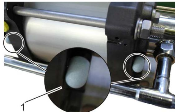
2. ➔ Connect the leak pipe (1) to the leak ports  $Z_1$  (2) and  $Z_3$  (3).
