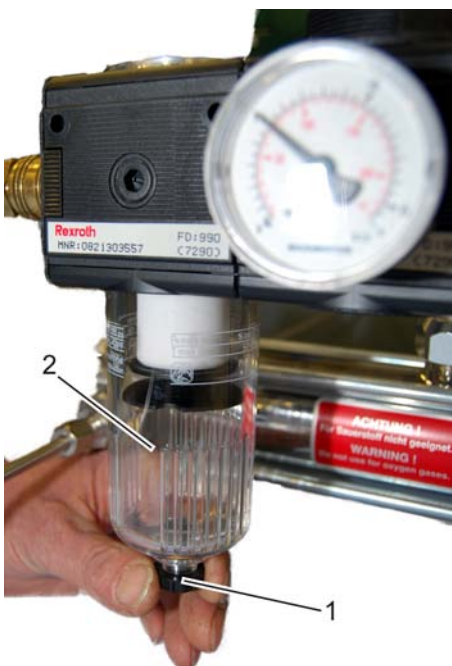
Fig. 25: Checking the water separator
