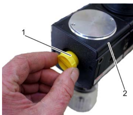
Fig. 9: Unscrewing sealing plug
