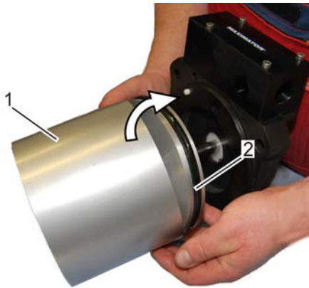
Fig. 71: Putting on the air cylinder
