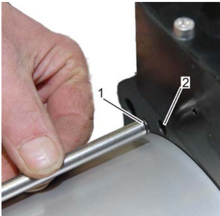
Fig. 77: Inserting the control tube
