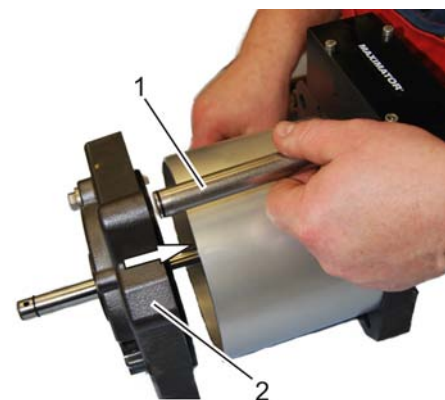
Fig. 78: Installing air pipes and lower cap
