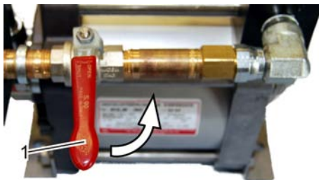
Fig. 24: Opening the ball valve
