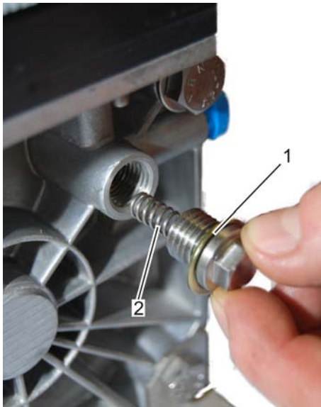
Fig. 46: Removing the threaded union
