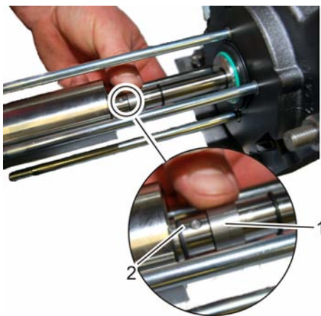
Fig. 80: Securing the dowel pin
