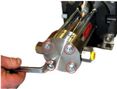
Fig. 54: Releasing the booster head
