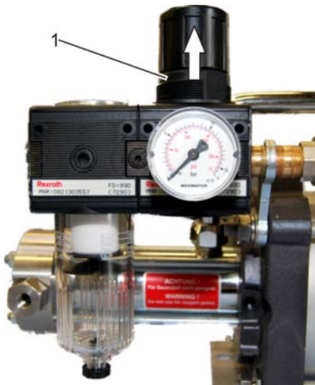
Fig. 22: Releasing pressure regulator from arrest
