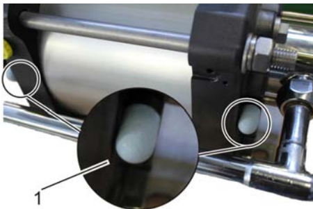
Fig. 12: Removing breather silencer
