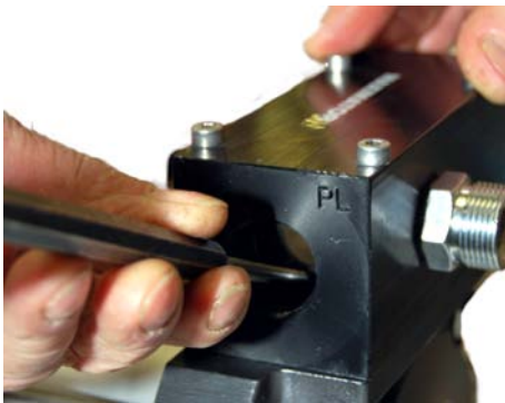
Fig. 39: Punching out the sleeve
