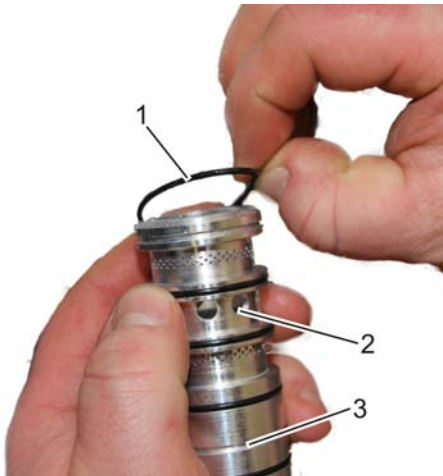
Fig. 41: Detaching the O-rings
