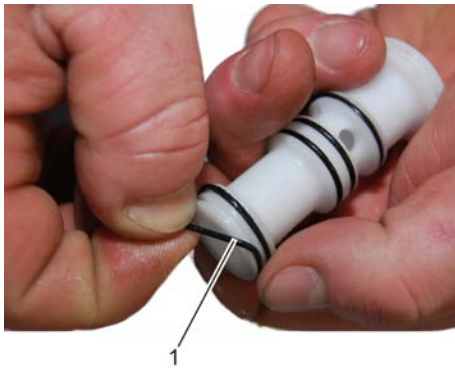
Fig. 32: Sliding on new O-rings
